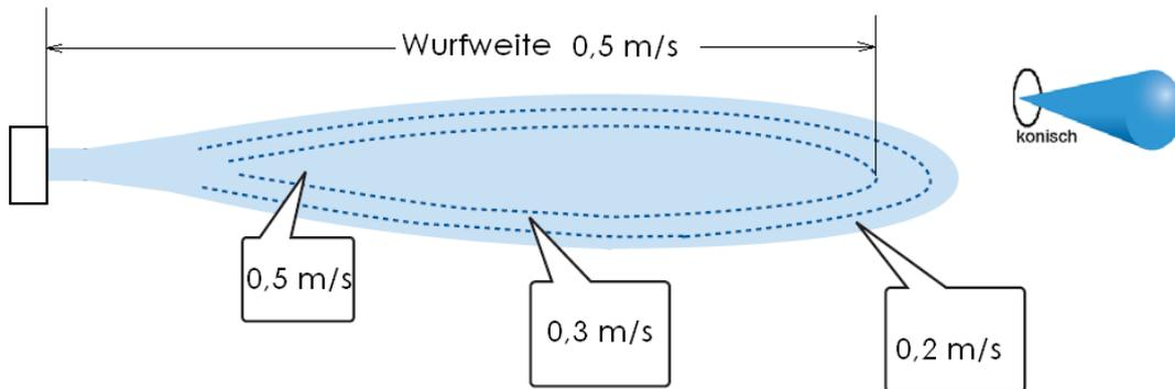
Figure 1: Definition of the air throw of an air cooler
