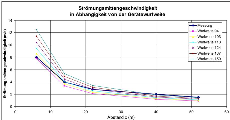
Figure 14: Comparison measurements / calculations
