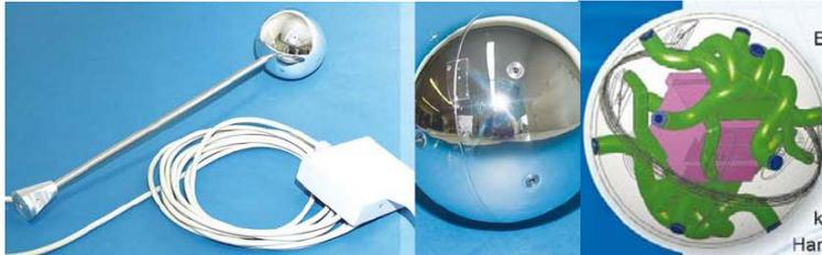
Figure 11: Measuring sensor of the 3D measuring system
