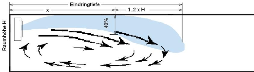
Figure 8: Separation point X and effective penetration depth
