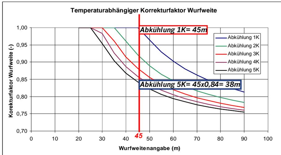
Figure 6: Influence of air cooling on air throw with a defined air cooler.
