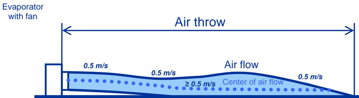
Figure 2: Measurement of air throw with previously used procedures
