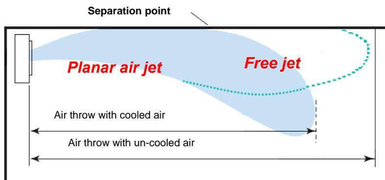
Figure 5: Consideration of Coanda effects and air cooling in air spread calculation of air throw
