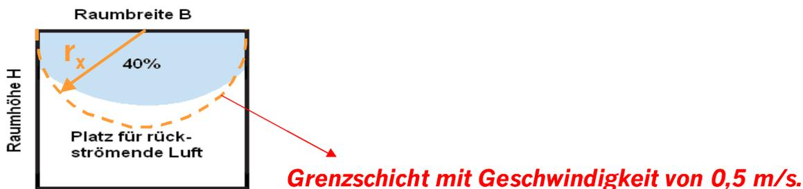
Figure 7 Room cross-section in air direction
