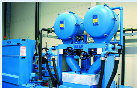
A cooling unit used to be fitted to every cutting oil - preparation centre. Now the cutting oil is cooled using a plate heat exchanger and a 17/24 °C cold water system.
