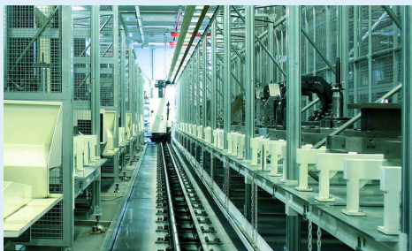
CNC machining in a group improves machine utilization and allows around-the-clock production.
